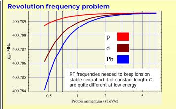
Compensate different speeds by adjusting closed orbit length.
