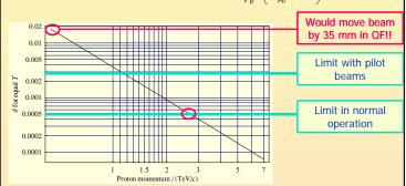
Revolution frequencies must be equal for collisions. Hard lower limit on energy of p-Pb collisions, Ep=2.7 TeV Energy where RF frequencies can become equal in ramp. Beam-beam encounters move at
