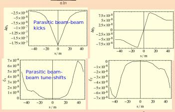
Assumes Pb ion bunch with nominal intensity  $N_b = 7 \times 10^7$ , proton bunch with 10% nominal intensity  $N_b = 1.15 \times 10^{10}$ , nominal emittances (equal geometric beam sizes).
