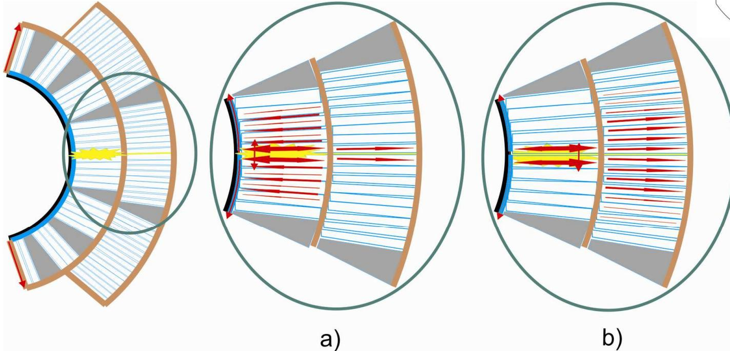
A sketch of the heat transfer in the magnet at nominal operation (a) and at quench limit (b).
