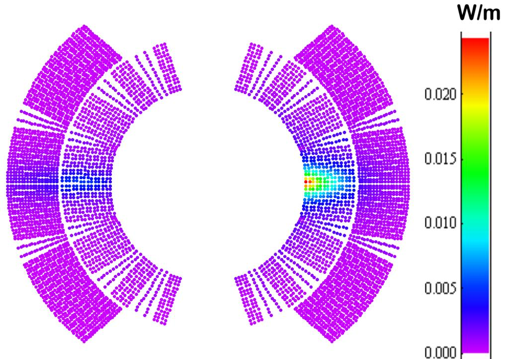
**Energy peak in the coil = 24.3 mW/m**
