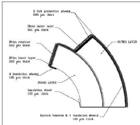
**Electrical insulation is the largest thermal barrier at 1.9 K against cooling**
